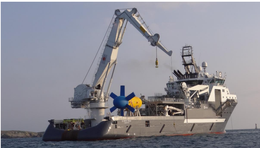
D10-1000 onboard Olympic Zeus after the lifting operation on the morning of April 11 th (@SABELLA / Région Bretagne)
